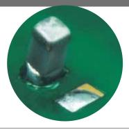
Offset Placement After Solder Screen-printing is a complete mounter solution promoting a self-alignment effect for reducing the rate of defects after reflow caused by solder printing positioning misalignment.
